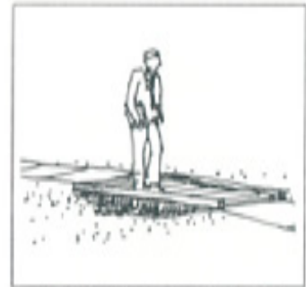
Simple wood plank bridge
